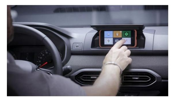
Most car manufacturers spend considerable time, effort and money to develop or source infotainment systems that typically feature a screen either integrated into the central dashboard, mounted atop the dashboard, or in fancier cars, under a single pane of glass.
