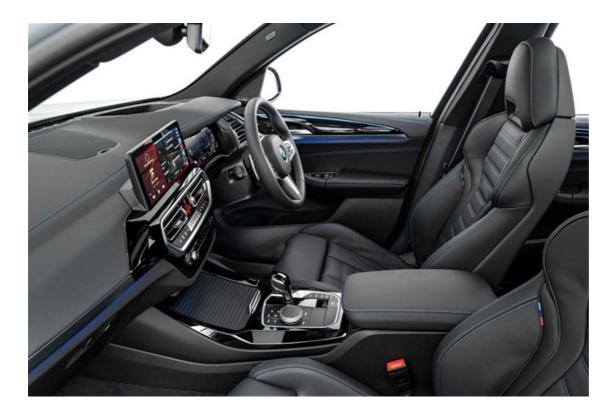
The centre console accommodates the newly designed control island with the gear selector lever, buttons for the start/stop system, the electric parking brake, hill descent control and various driving experience functions as well as the BMW Controller. The engine start button is positioned here, too.
