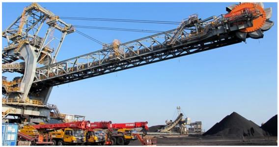
One of the two new rail-mounted stacker reclaimers which scoop up and transfer coal into and out of the yard is seen at Africa's largest coal export facility, the Richards Bay Coal Terminal, 2018. Source: Reuters/Tanisha Heiberg
