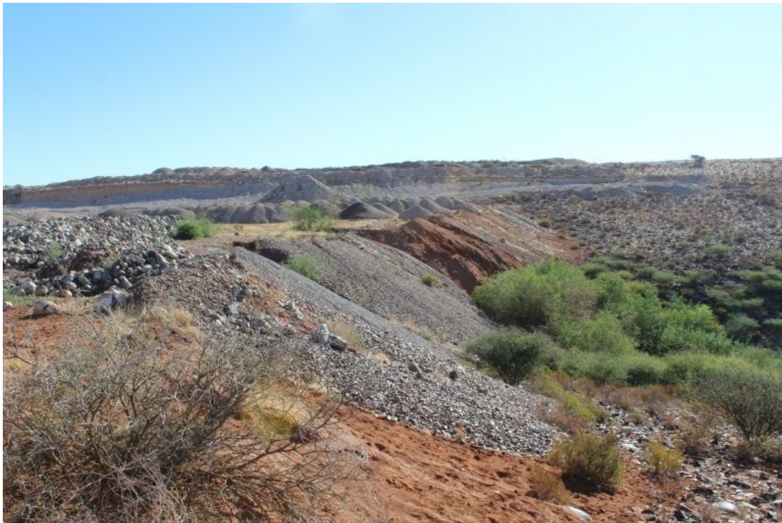
Regulations make it mandatory for mined gravel to be returned. In this case, the gravel is poured into the watercourses, from where it will be shifted, after a little rain, to the Orange River.
