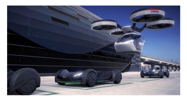
For megacity journeys, the capsule disconnects from the ground module and is carried by a 5m x 4.4m air module propelled by eight counter-rotating rotors. In this configuration, Pop.Up becomes a self-piloted air vehicle, taking advantage of the third dimension to get from A to B while avoiding traffic congestion on the ground.
