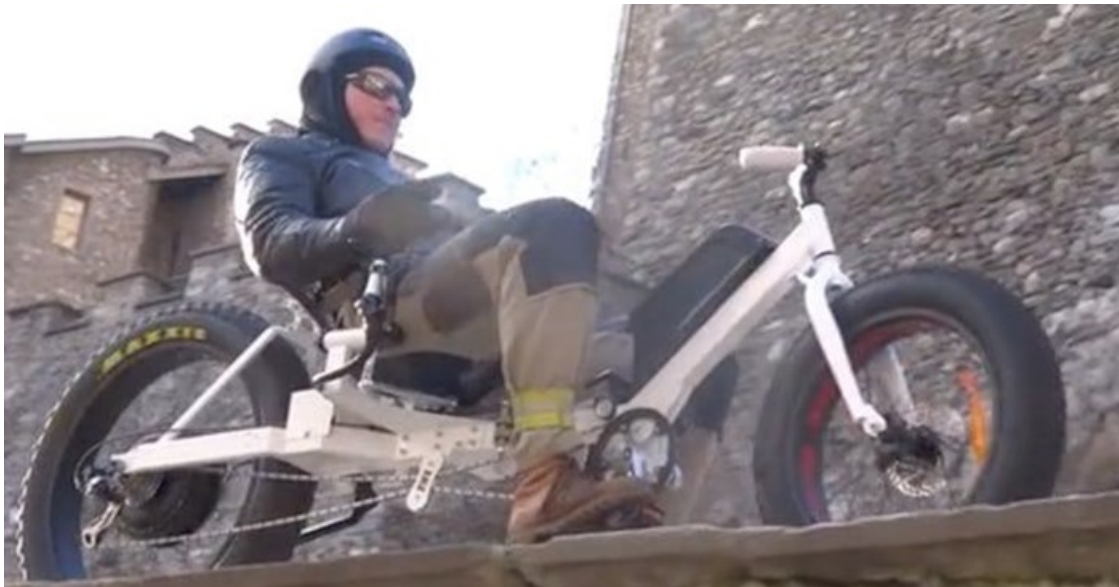
The Joystickbike ditches the handlebars in favor of a joystick (Credit: Joystickbike)
