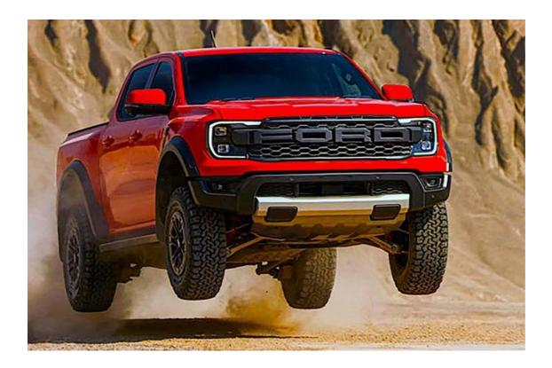
Ford Performance ensured the engine delivers immediate response to throttle inputs, and a race-bred anti-lag system, available in the Baja drive mode, enables rapid delivery of boost on demand by keeping the turbochargers spinning for up to three seconds after the driver backs off the throttle.
