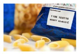
Ideal for flexible packaging, thermal transfer overprinting (TTO) is a digital printing process that has largely replaced hot stamping and other more traditional analogue printing techniques, largely because of its cost reduction.
