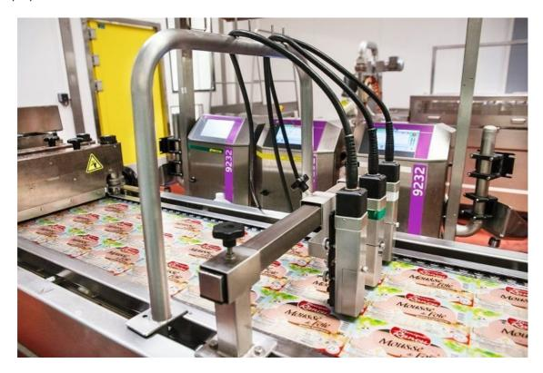
And, when it comes to coding flexible film, companies are turning away from mechanical technologies, such as hot stamping and rotary coding, in favour of four digital options that improve traceability and uptime: thermal transfer overprinting (TTO), continuous inkjet (CIJ), thermal inkjet (TIJ) and laser marking.
