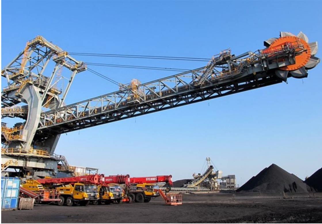
One of the two new rail-mounted stacker reclaimers which scoop up and transfer coal into and out of the yard is seen at Africa's largest coal export facility, the Richards Bay Coal Terminal, Richards Bay harbour, South Africa, June 21, 2018. REUTERS/Tanisha Heiberg
