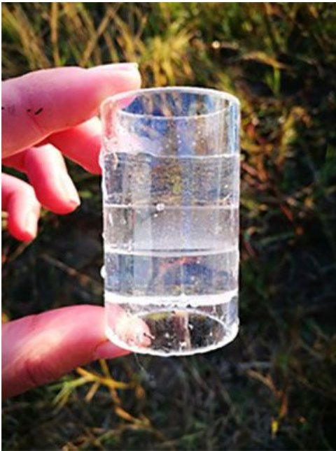
The artificial mussel developed by NWU and UDE researchers to monitor platinum in fresh water
