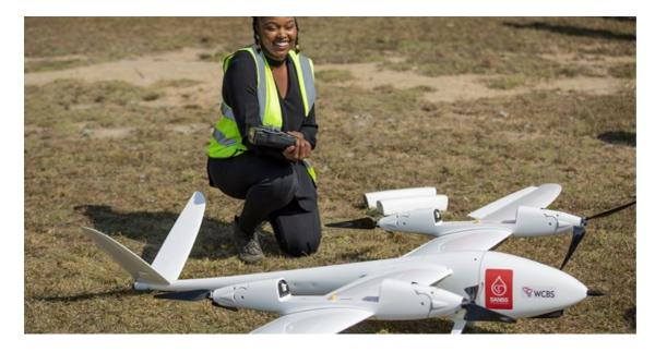
The Tron unmanned aerial vehicle (UAV) is a highly specialised aircraft capable of vertically taking off and landing, which can transport blood much faster and more efficiently than ever before.
