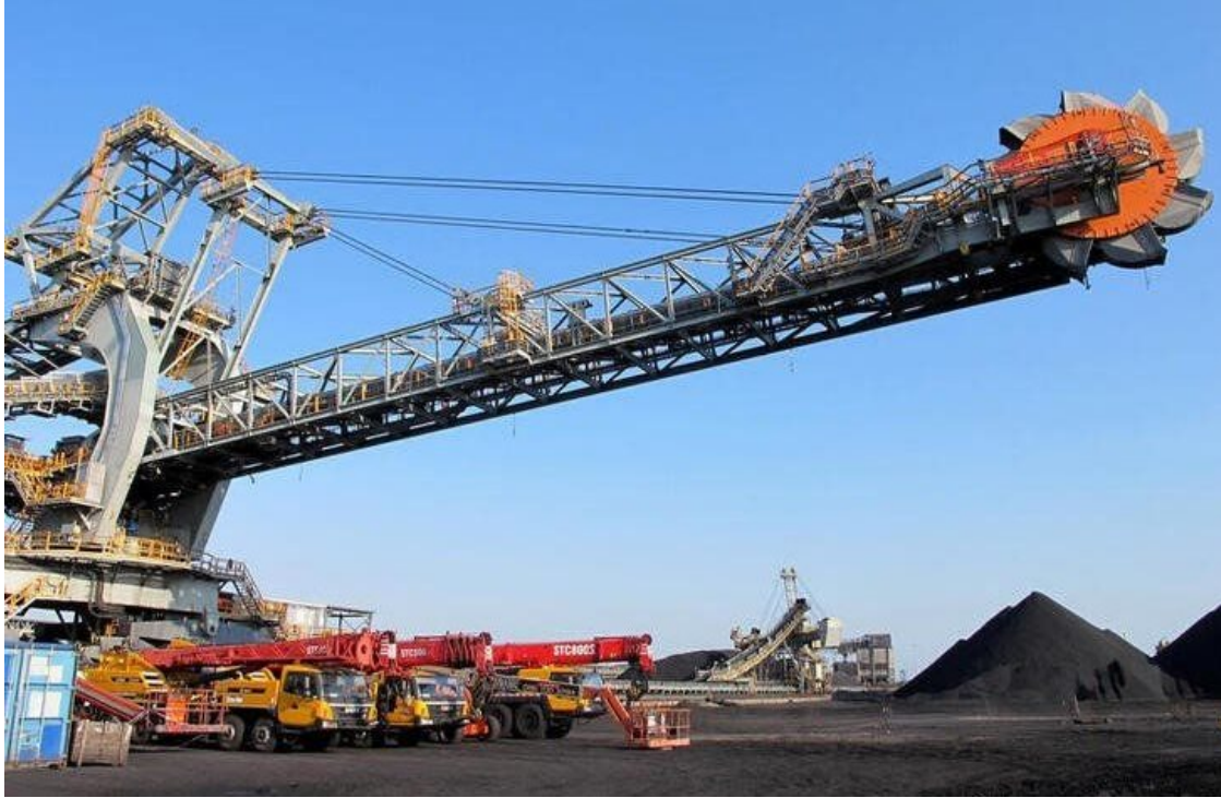
One of the two new rail-mounted stacker reclaimers which scoop up and transfer coal into and out of the yard is seen at Africa's largest coal export facility, the Richards Bay Coal Terminal, Richards Bay harbour, South Africa, June 21, 2018. REUTERS/Tanisha Heiberg/File Photo
