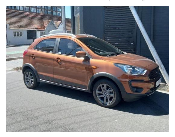
The Freestyle has a three-cylinder 1.5-litre petrol engine that provides 91kW of power and 150Nm of torque to the front wheels through a manual transmission.
